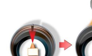
8. The inside surface of the weld is sprayed with lacquer and then cured by blowing heated air onto the outside of the cans.
