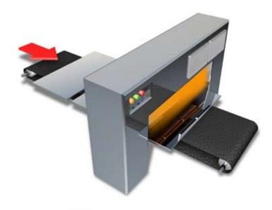
5. The large sheets are slit into small sheets, one for each can body.
